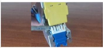
Squeeze handles together terminating and trimming wires
