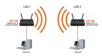
Connecting two separate LANs together through two DAP-1360 units (Wireless PCs cannot access the DAP-1360 units)
