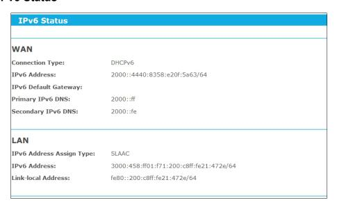
The **IPv6 Status** page displays the router's current IPv6 status and configuration. All information is read-only.
