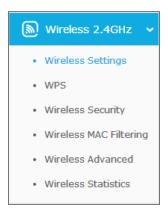
There are six submenus under the Wireless menu, shown in the figure above **Wireless Settings**, **WPS**, **Wireless Security**, **Wireless MAC Filtering**, **Wireless Advanced** and **Wireless Statistics**. Click any of them, and you will be able to configure the corresponding functions.
